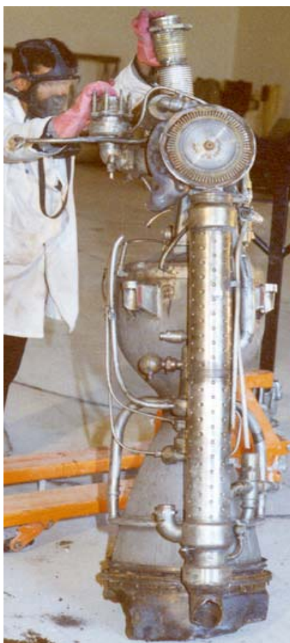
Figure IV.III.XXVI SCUD engine test using UDMH fuel and a nozzle extension skirt.
